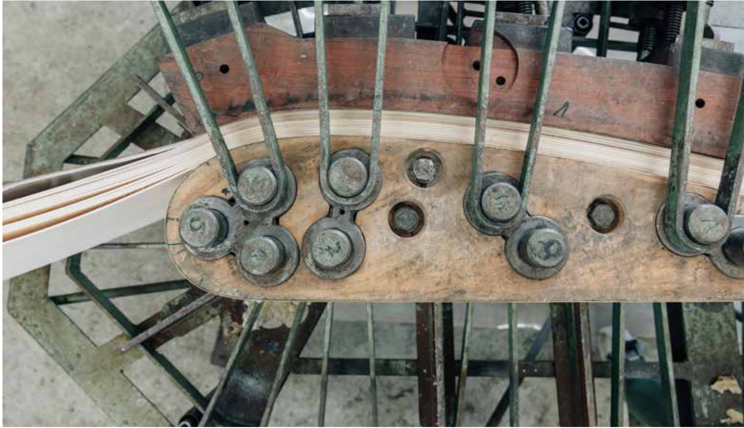
(No Model.) C. F. T. STEINWAY. Screw Clamp for Wood Bending Machines. No. 229,198. Patented June 22, 1880.
